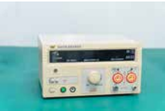
Voltage withstand test
